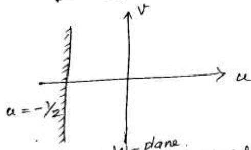
$\therefore$  The image of the circle  $|z|=1$  in  $z$ -plane is the straight line  $u = -\frac{1}{2}$  in  $w$ -plane under  $w = \frac{z}{z-1}$  or  $\frac{z}{1-z}$ .
